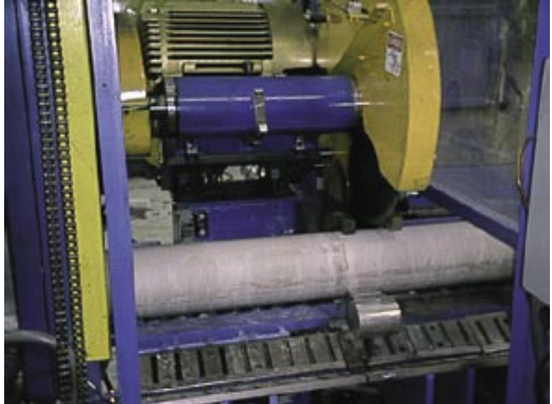
Hot Log Saw* cutting heated log to precise billet length
