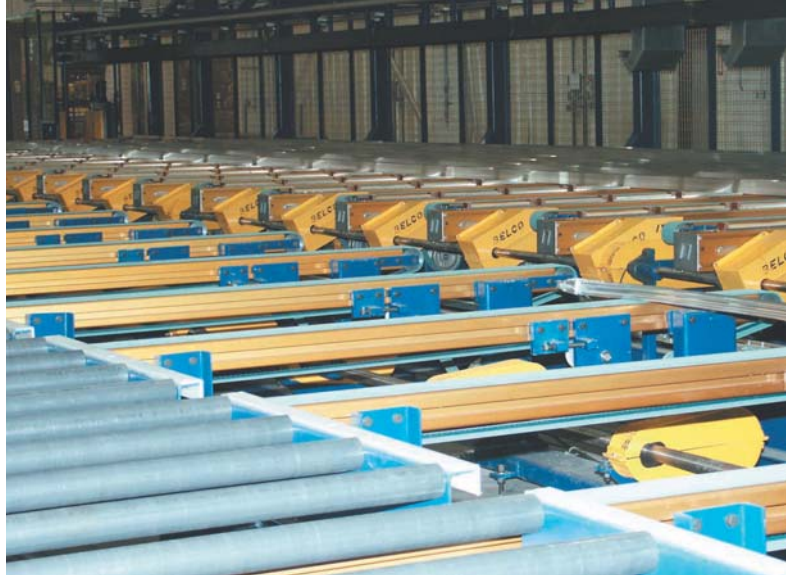
ROLT Cooling and Belt Storage Conveyors
